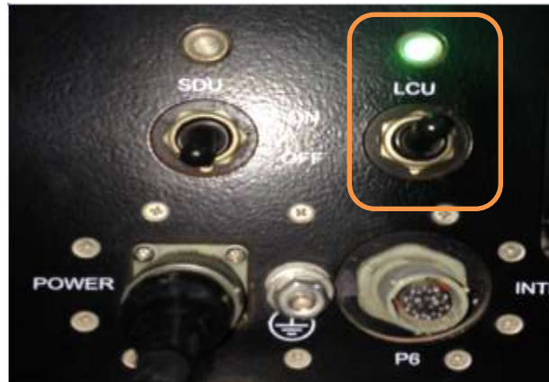
Figure 5 SDU power -SDU and LCU power switches
