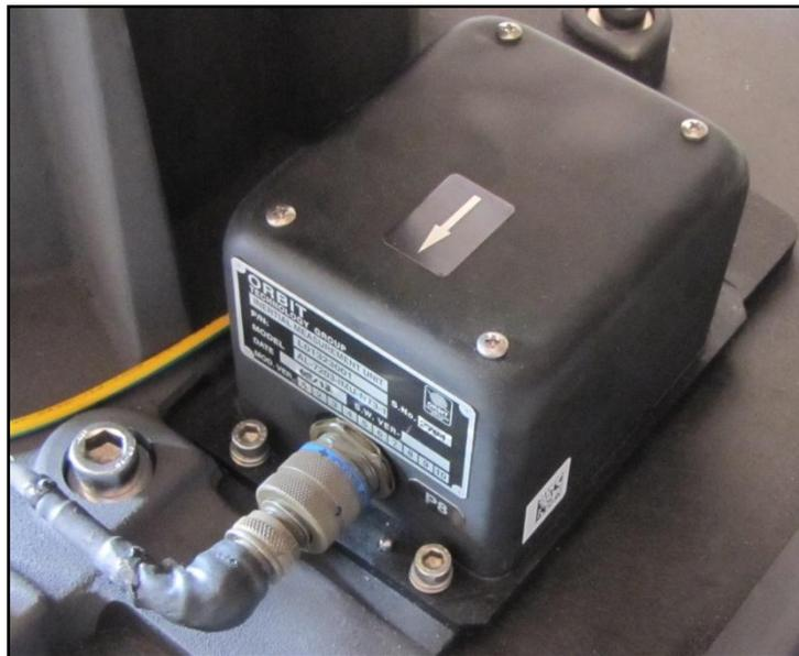
Figure 1-1: Inertial Measurement Unit
