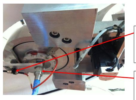
Secure the Rx Cable F-Type connector using tire up
