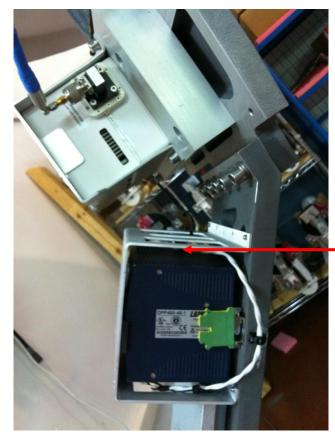
Secure the MOLEX connector of the <u>AC Input cable</u> and <u>DC output cable</u> (connected to the Power supply) properly to the Power supply cover.
