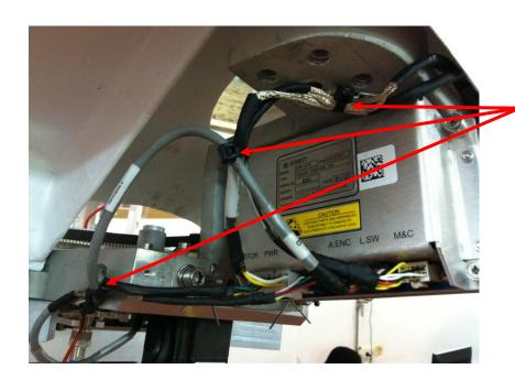
Secure the cables using a tire up
