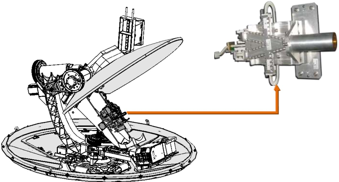
Figure 1-1 Ka Circular Feed and its location on the pedestal.
