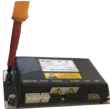
Figure 1-2 Release x4 Captive Screws
