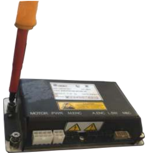
Figure 2-1 Release x4 Captive Screws
