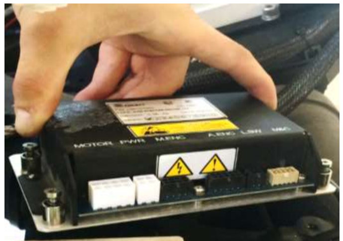
Figure 1-2 Release x4 Captive Screws
