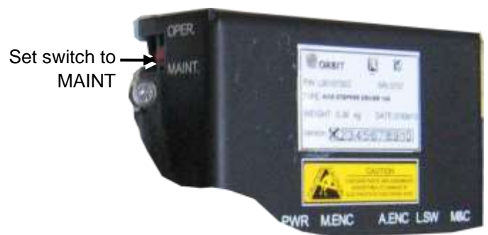
Figure 2-3. Verify switch is on MAINT
