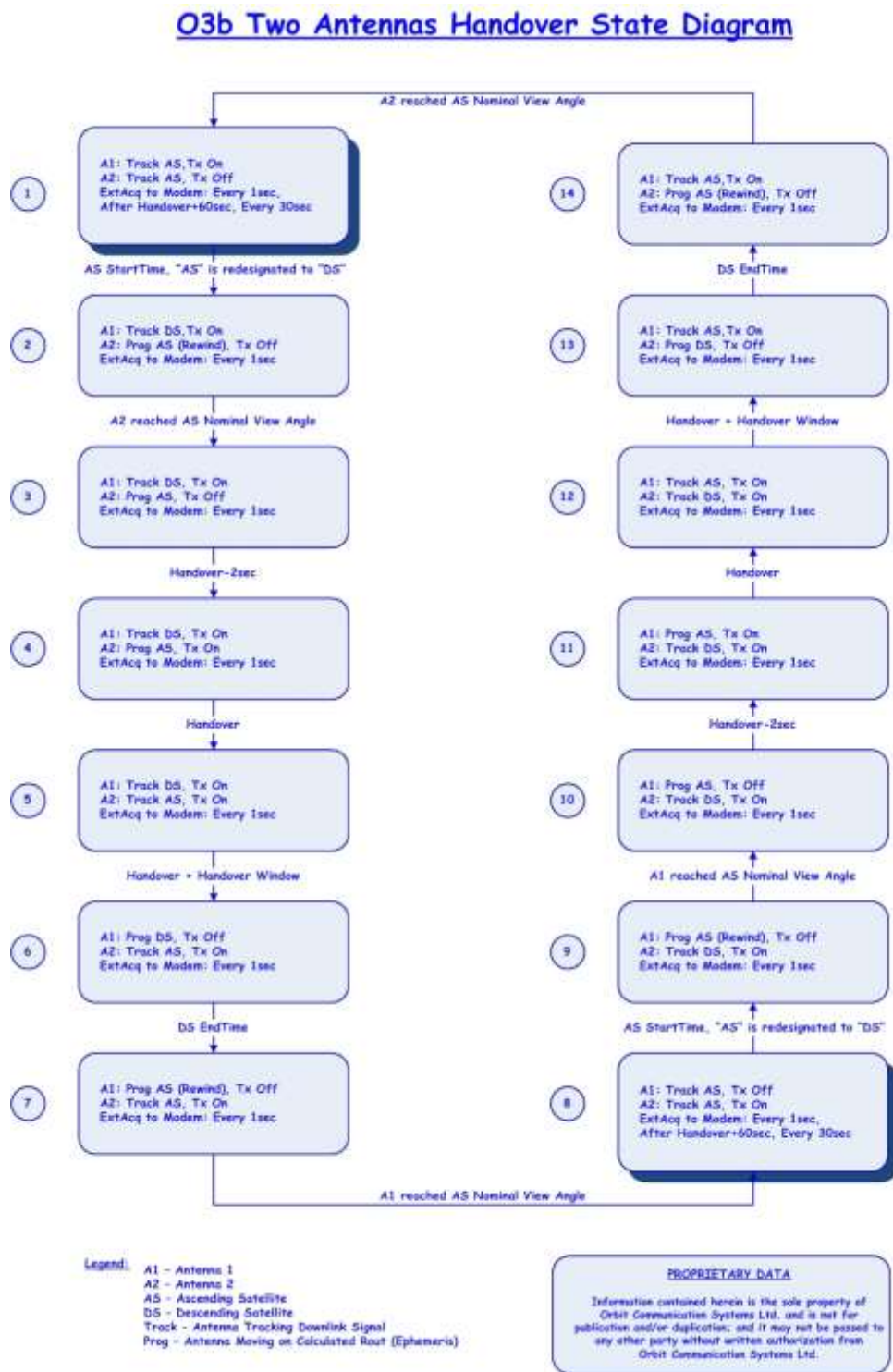
Figure 6-1: Handover Flow for Two Antennas
