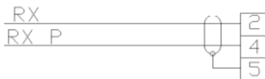
Figure 3-6: RS-422 NMEA-0183 Mating Connector Wiring Diagram
