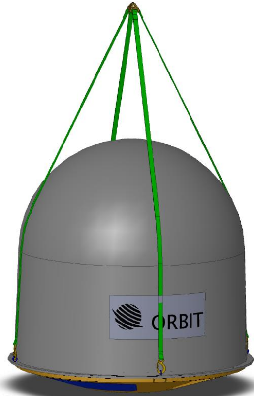
Figure 3-6: Harness lifting the unit
