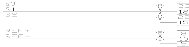
Figure 9-31: SYNCHRO Mating Connector Wiring Diagram
