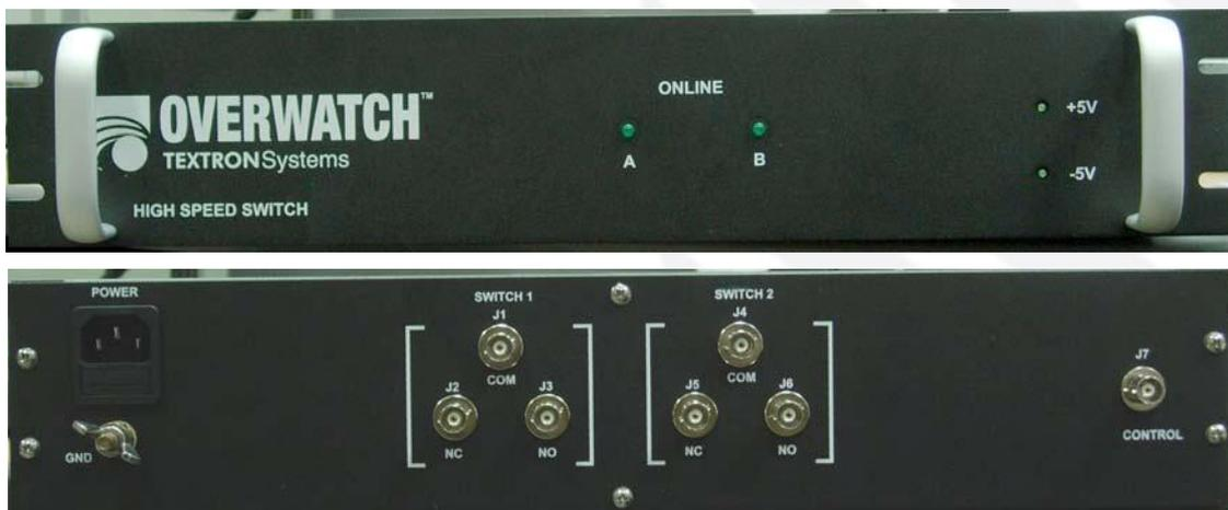
Figure 10 - IF Switch Connectors (Front and Rear Panels)
