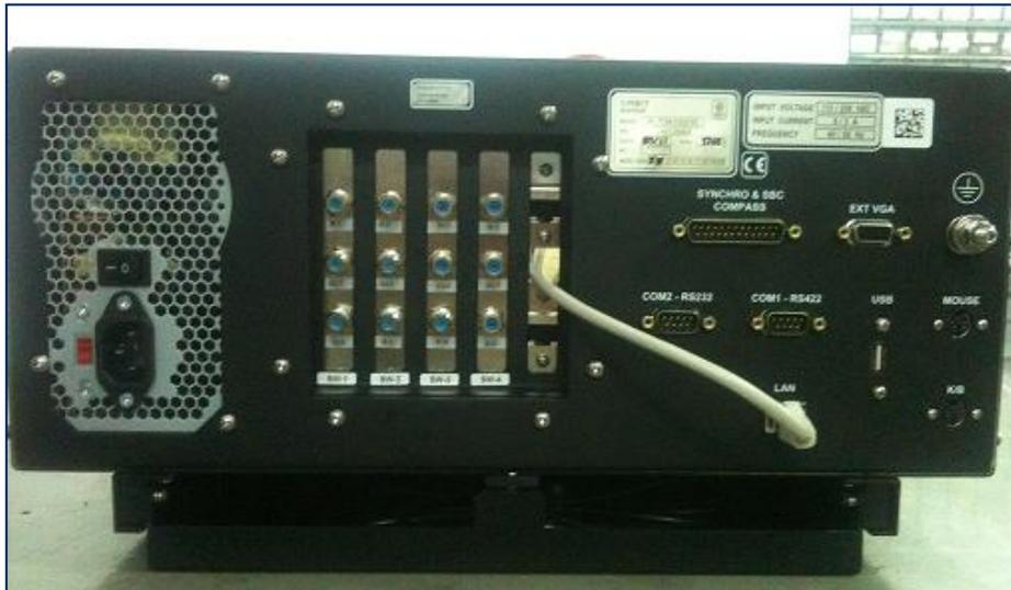
**Figure 6 - CCU Rear Panel Connectors (with LAN)**
