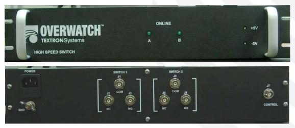
Figure 10 - IF Switch Connectors (Front and Rear Panels)
