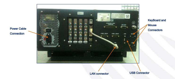
Figure 7 - CCU Rear Panel - General Purpose Connections
