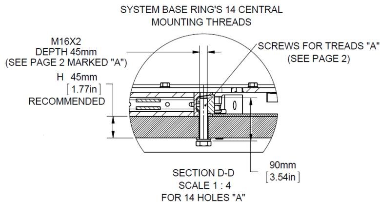
If necessary, use wide washers (supply as part of the ADE installation KIT) below the mast support structure to ensure that the bolts can be tightened properly.
