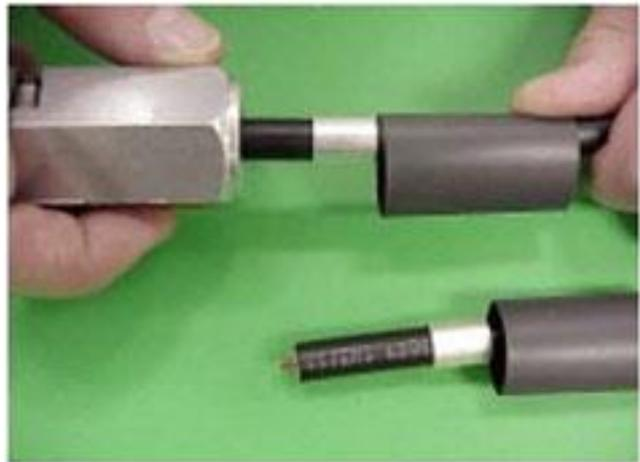
**STEP 3:** Insert the cable into End 2 of the ST-400-EZ prep/strip tool and rotate the tool to remove the plastic jacket.
