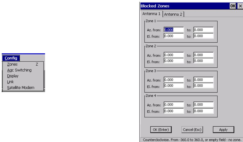
**Figure 11.9-5: Blockage Zones Window for DAO (Dual System Topology, CCU CE)**
