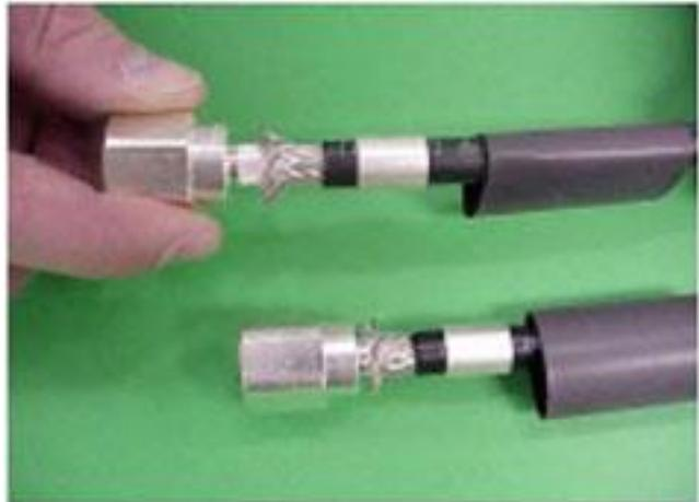
**STEP 6:** Temporarily slide the crimp ring back, and remove the connector body from the cable to trim the excess braid at the crease line, then remount the connector and slide the crimp ring forward until it butts up against the connector body.
