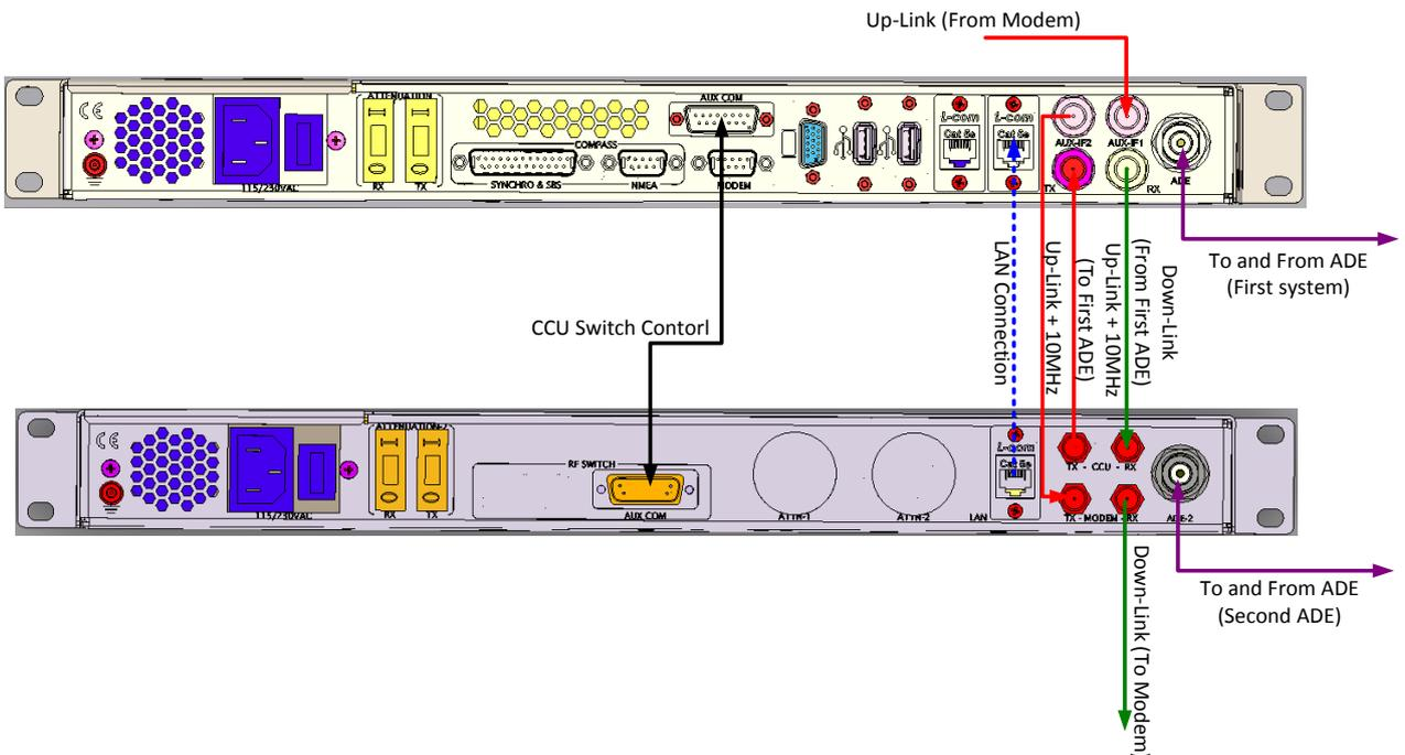
**For Orbit System Selector (OSS) configuration,** In case of using the 10MHz Signal reference from the Modem Up-Link (Tx) port, the following connection set up can be used:
