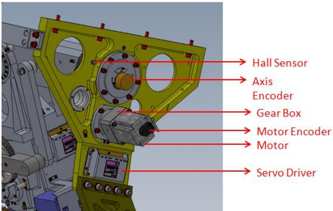
Figure 6.5-2: Servo-Sub-System components
