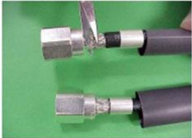
**STEP 7:** Position either the heavy duty HX-4 crimp tool with the appropriate dies (0.429" hex) or the CT-400/300 crimp tool directly behind and adjacent to the connector body and crimp the connector. The HX-4 crimp tool automatically releases when the crimp is complete.
