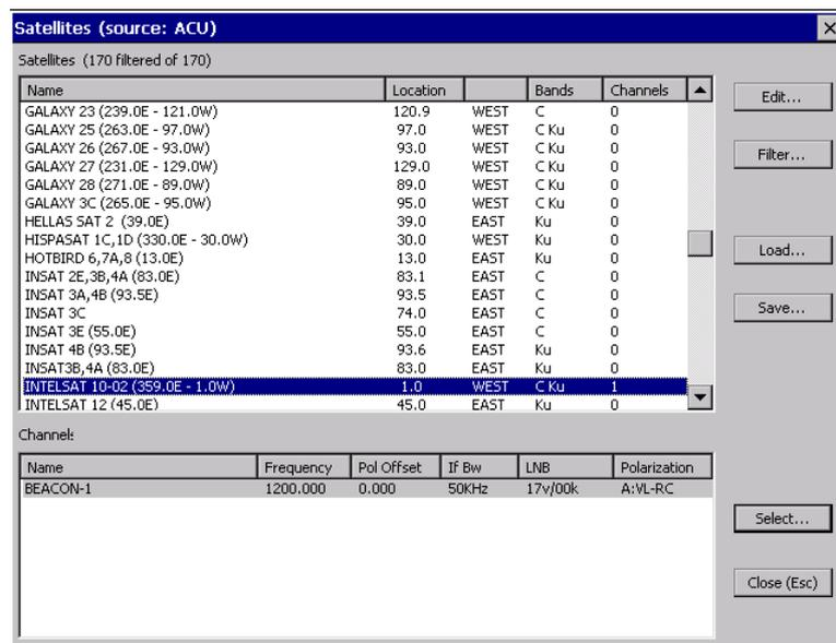
Figure 11.5-1: GEO Satellites Database window
