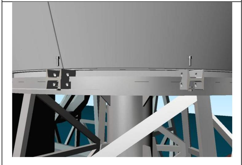
**STEP 5:** Insert M16 bolts washers and spring washers upwards through the system support and into the 14 threaded holes in the center of the ADE Base Ring.
