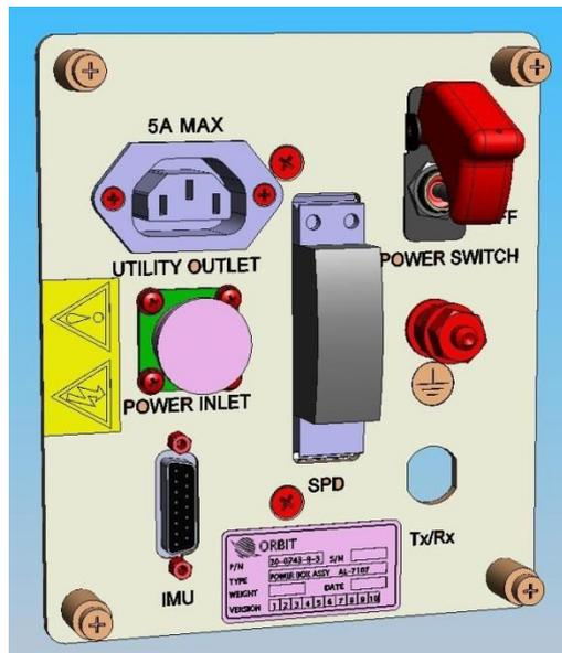
Figure 6.3-1: ADE Antenna Power Connections BOX
