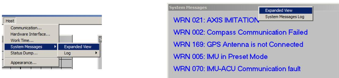
**Figure 12.15-3: Message Log Window – Expanded View**
