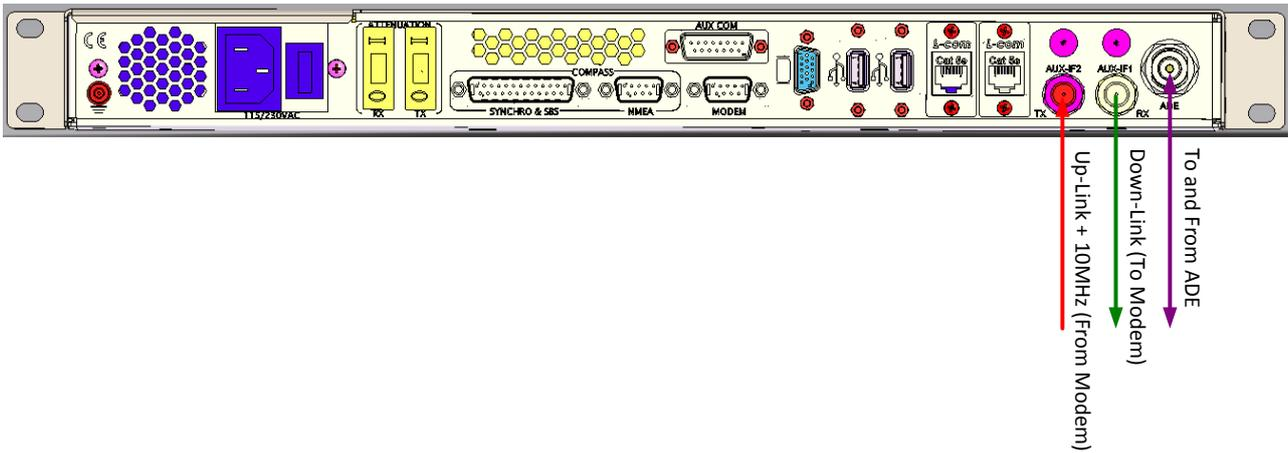
In case that the 10MHz Signal reference is not supplied from the Modem Up-Link (Tx) port, the following connection set up can be used:
