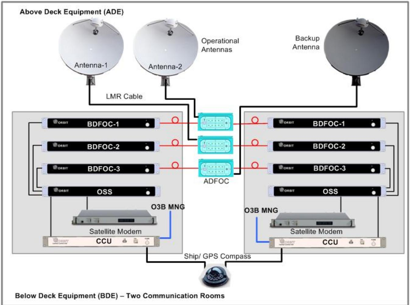
Figure 2.5-1: Dual room Configuration Architecture Overview
