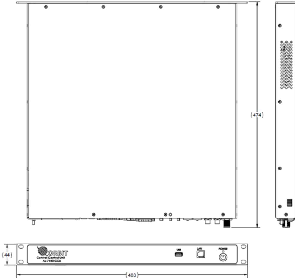
**Figure 8.5-1: CCU/DSS/OSS 1U Mechanical Dimensions**
