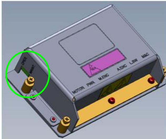
Figure 9.4-1: Servo Driver OPER and MAINT Switch
