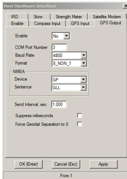
**Figure 12.11-1: Host Hardware- GPS Output tab**
