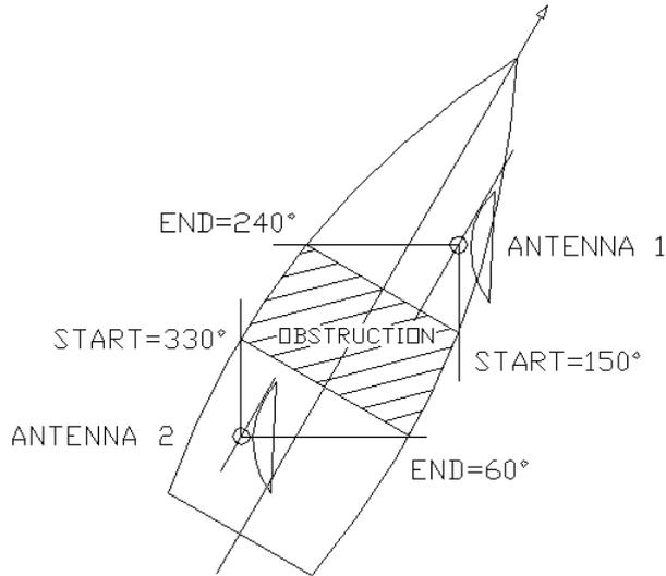
**Figure 11.9-3: Blockage Zone Example**
