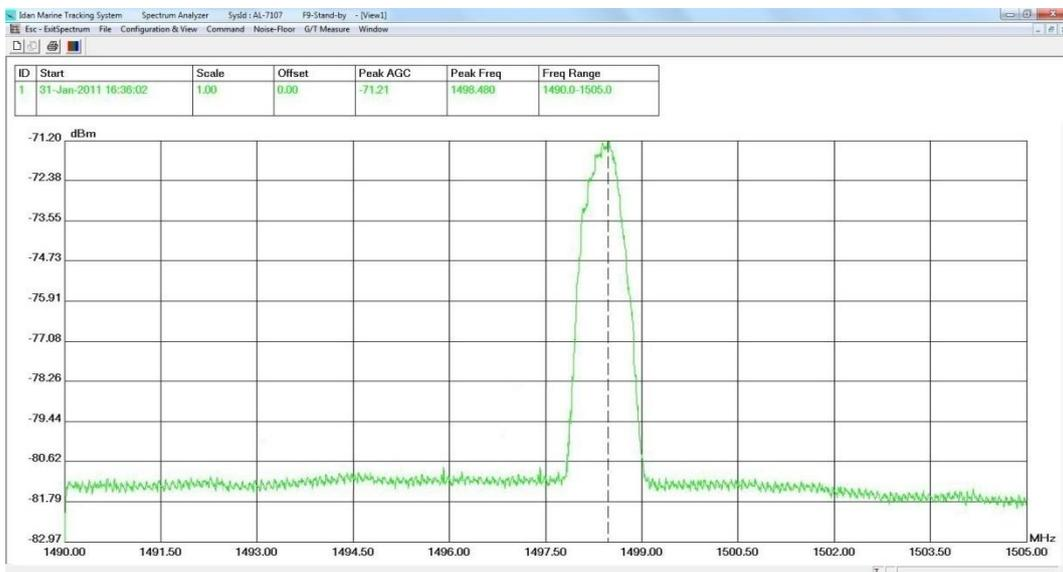
**Figure 12.19-4: MtsVLink Spectrum Analyzer Display with an NBR IfBw of 150 KHz**
