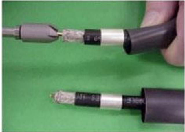
**STEP 5:** Flare the braid slightly and push the connector body onto the cable until the connector snaps into place, then slide the crimp ring forward, creasing the braid.
