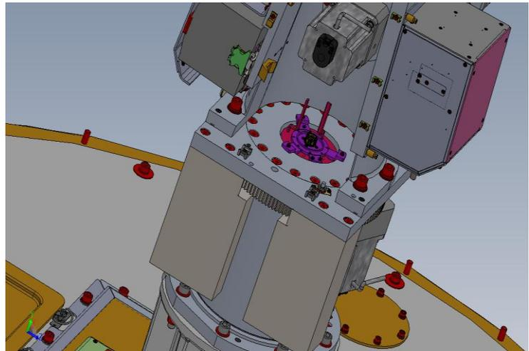
Figure 6.4-1: Slip-Ring/Rotary-Joint Assembly
