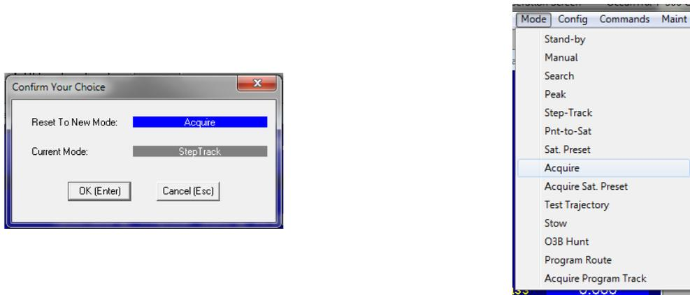
**Figure 11.6-1: Setting the ADE Antenna to Acquire Mode**
