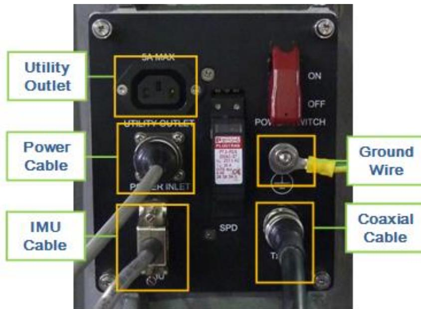
Figure 10.2-1: ADE Antenna Power Connection BOX Cables
