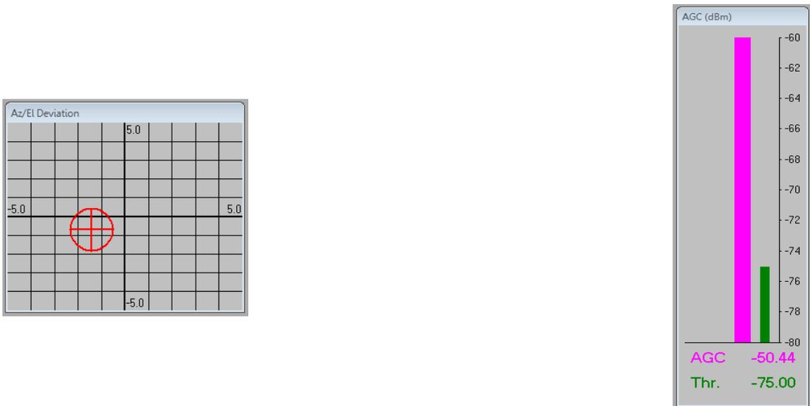
**Figure 11.6-6: AGC Signal Acquired before Compass Offset adjustment**
