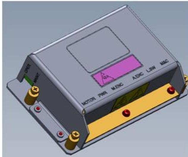
**Figure 6.5-3: Axis Servo-Driver**
