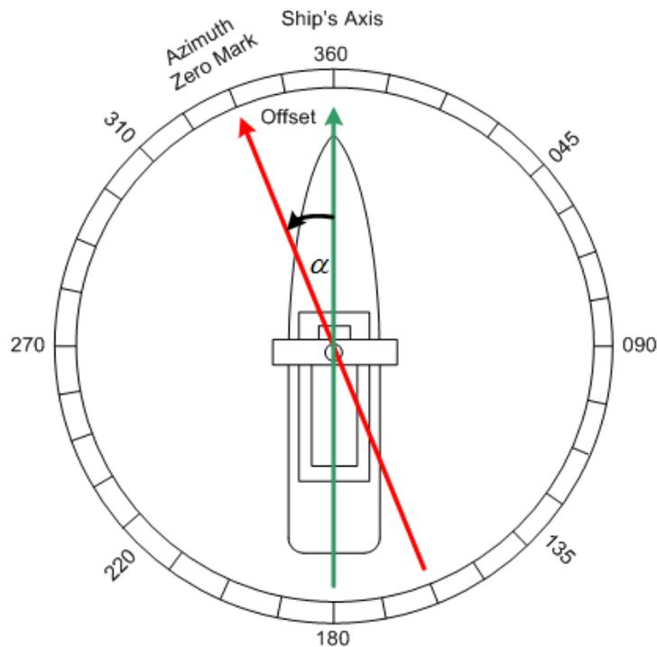
**STEP 5:** Enter a preliminary compass **Offset** value. (This will be updated during the Compass Offset procedure).
