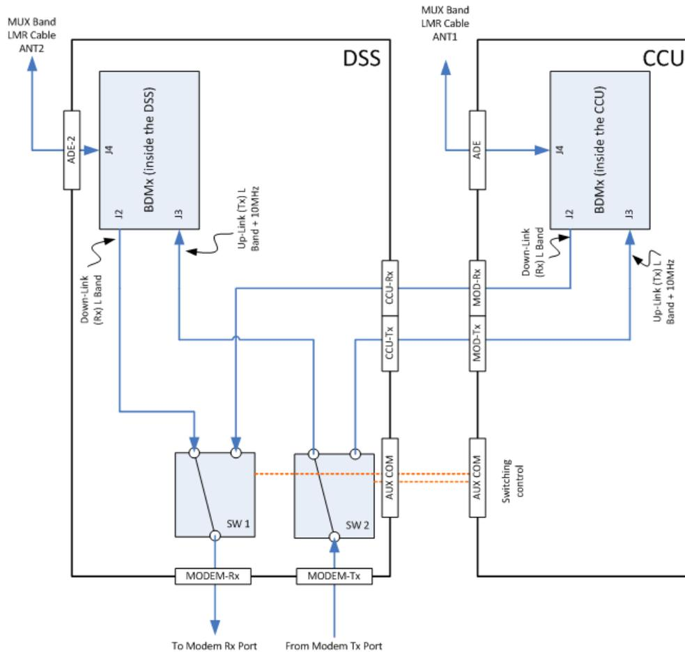
**Figure 7.2-1: DSS Switching Scheme**
