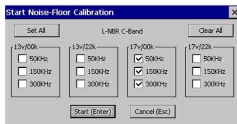
**Figure 12.6-2: Start Noise-Floor Calibration Dialog Box**
