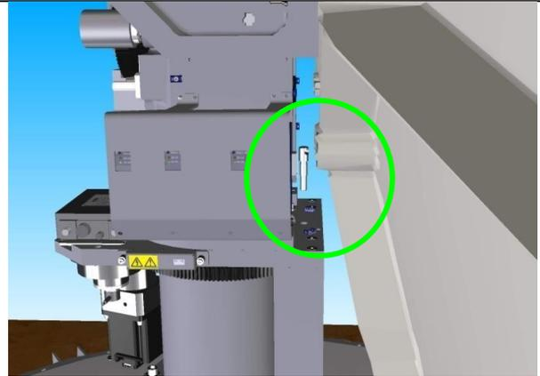
**Figure 9.3-3: Azimuth Stow Lock Pin**
