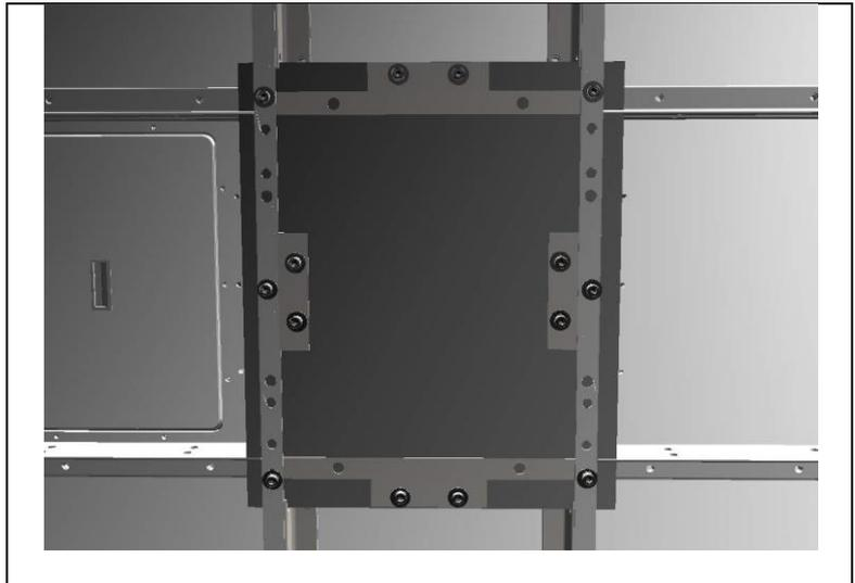
The 14 bolts that attach the center of the ADE Base Ring to the mast support structure should not protrude more than 45mm from the mast support structure top plate level due to the ADE Base Ring threads depth of 45mm.
