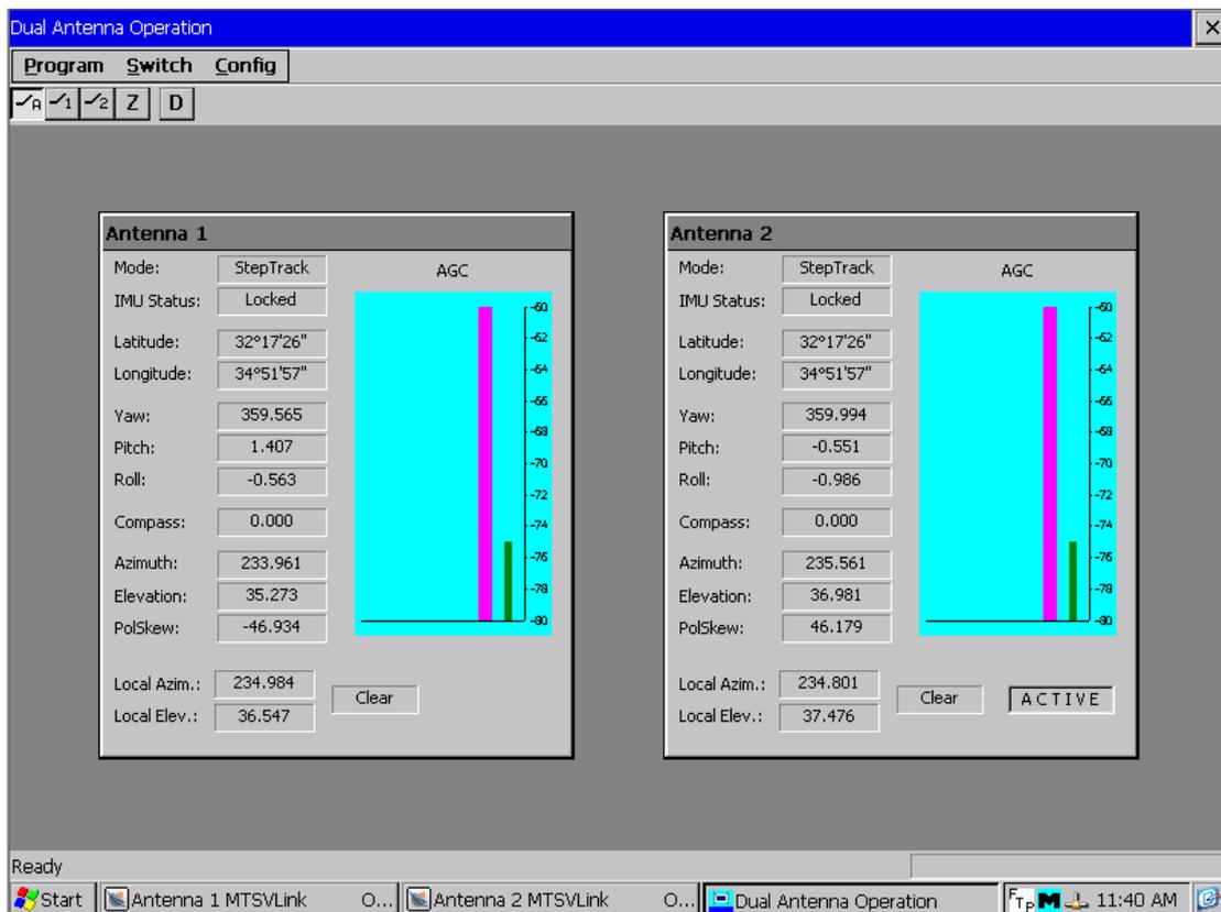
Figure 5.3-1: DAOLink Main Screen
