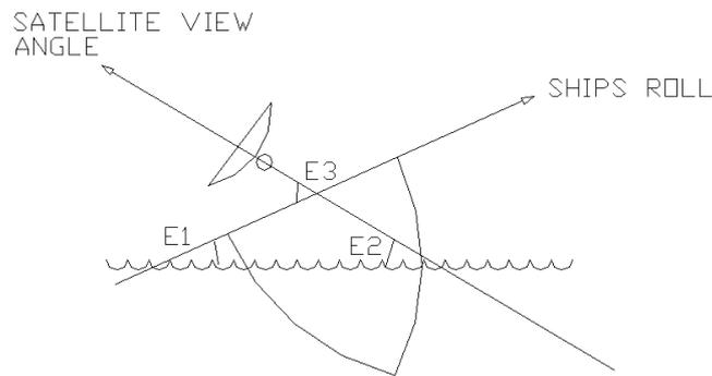
**Figure 11.9-2: Blockage Zone Elevation Variables**
