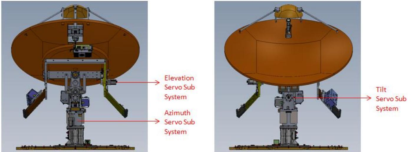
Figure 6.5-1: Azimuth, Elevation and Tilt Servo-Sub-Systems
