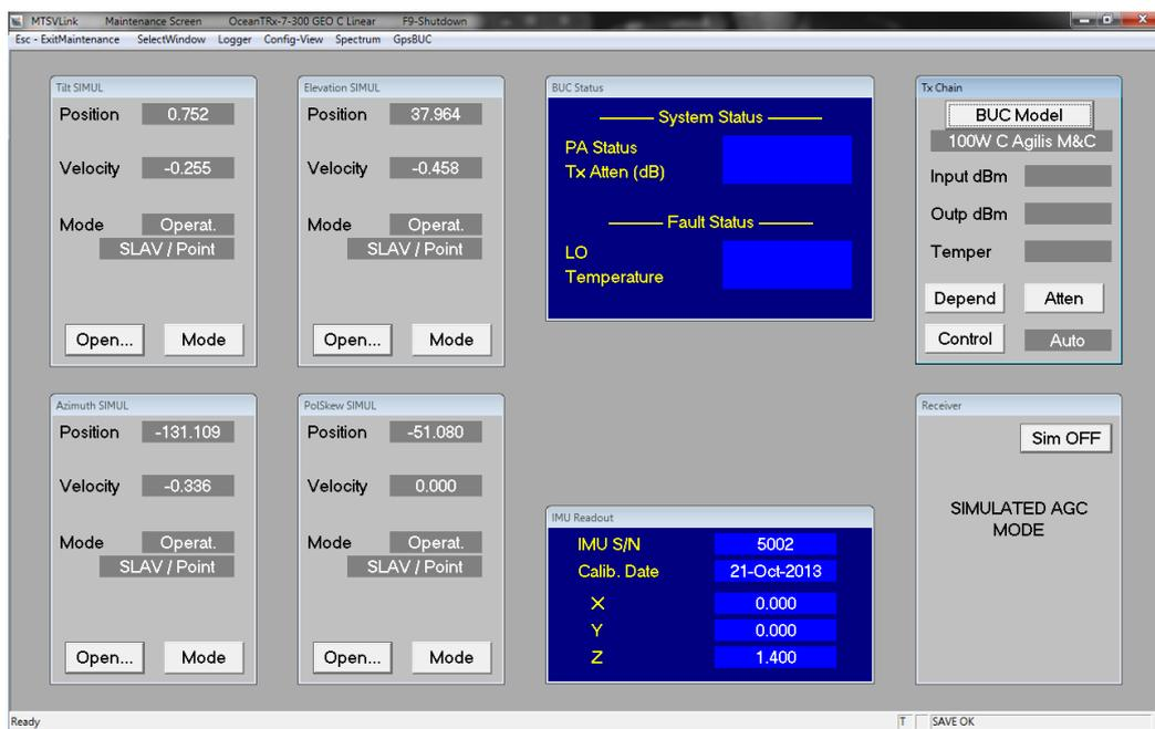
Figure 11.10-1: BUC Tx Chain and Status Windows uses for Monitor and Control
