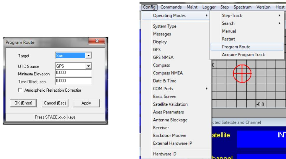
Figure 11.6-3: Setting the ADE Antenna Program Route Target to SUN
