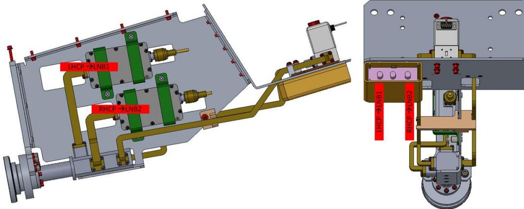
Figure 6.7-1: OceanTRx™7-500 Ka Circular Feed and LNB Mounting
