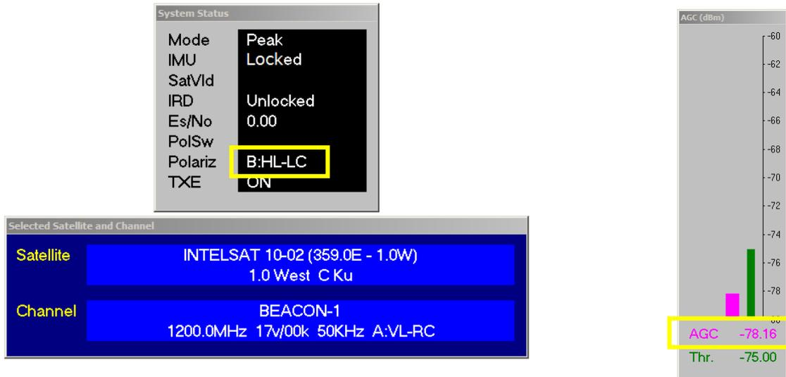
Figure 11.7-4: AGC Signal received level at X-Polarization before offset
