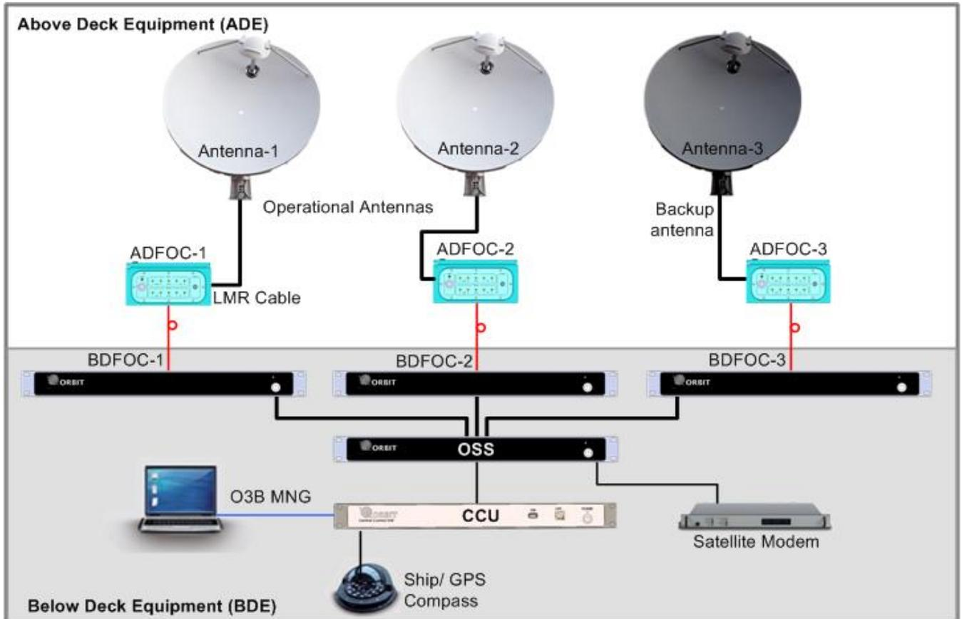
Figure 2.4-1: Single room Configuration Architecture Overview
