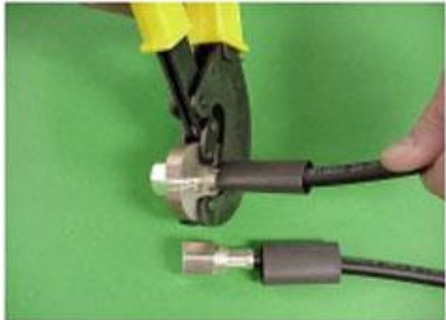
**STEP 8:** Position the heat shrink boot as far forward on the connector body as possible without interfering with the coupling nut and use the heat gun to form a weather-tight seal.
