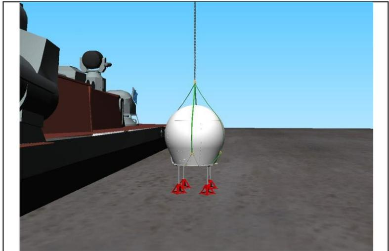
**STEP 2:** Attach the anchor shackles at the end of each short strap to the *right hole* in 8 of the 10 lifting points protruding from the ADE Base Ring.
