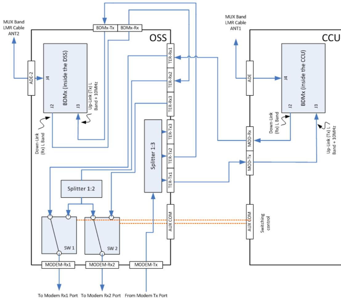
Figure 7.3-1: OSS Switching Scheme
