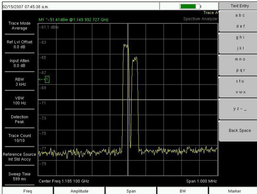
**Figure 12.19-2: Anritsu MS2721A Spectrum Analyzer Display with a 3 KHz RBW**
