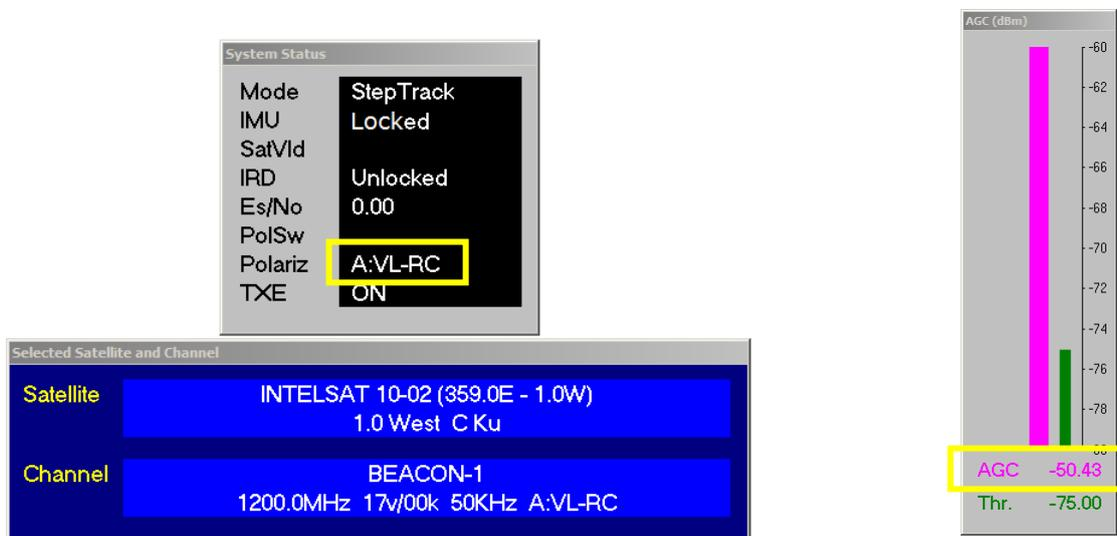
**Figure 11.7-2: AGC Signal received level at Co-Polarization**
