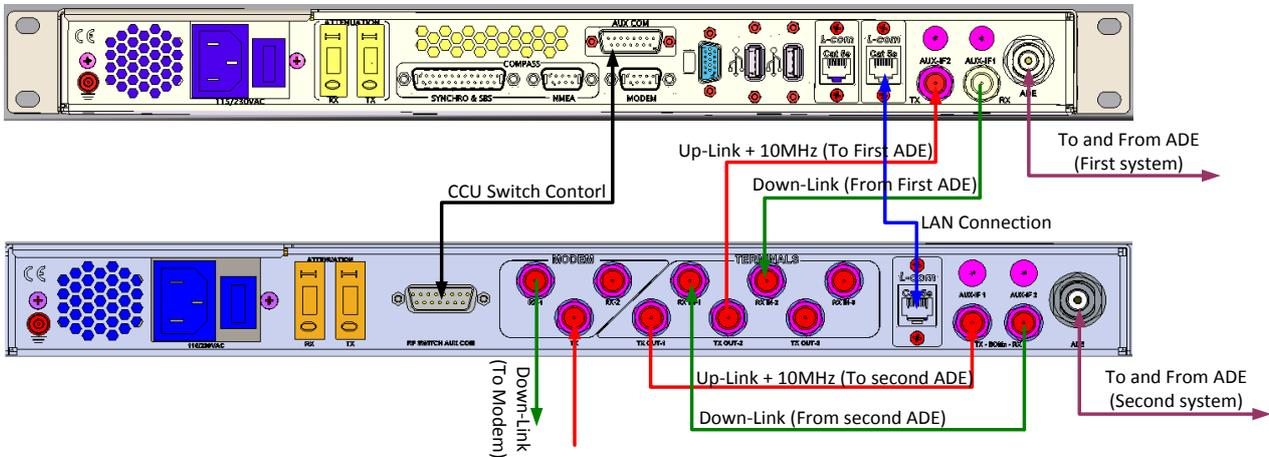
**For Orbit System Selector (OSS) configuration,** In case that the 10MHz Signal reference is not supplied from the Modem Up-Link (Tx) port, the following connection set up can be used:
