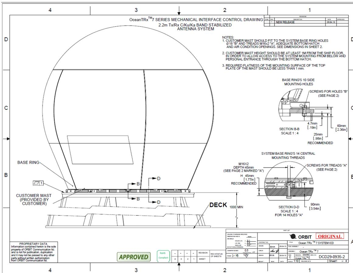
Figure 8.1-1: OceanTRx™7 Interface Control Drawing (Mechanical)
