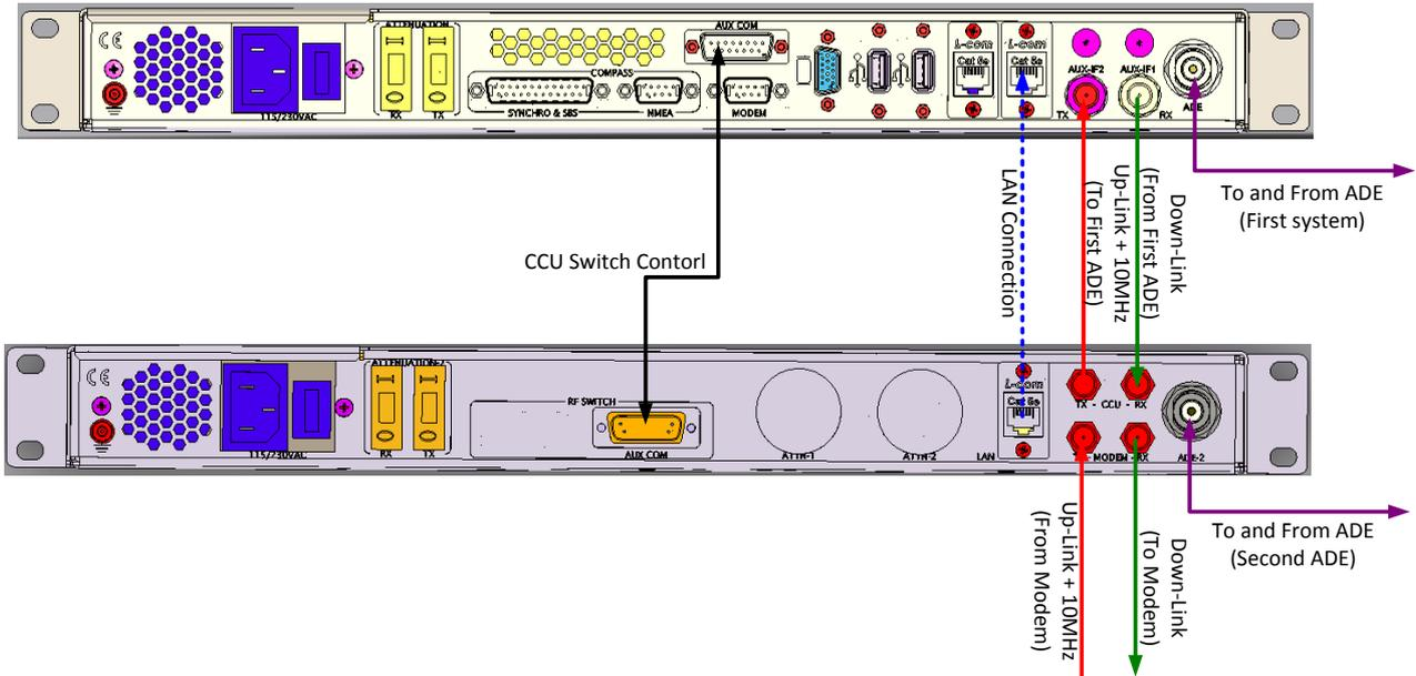
**For Dual System Selector (DSS) configuration,** In case that the 10MHz Signal reference is not supplied from the Modem Up-Link (Tx) port, the following connection set up can be used:
