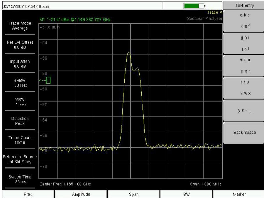
**Figure 12.19-3: Anritsu MS2721A Spectrum Analyzer Display with a 30 KHz RBW**
