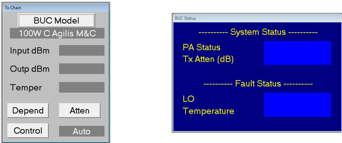
Figure 11.10-2: BUC Tx Chain and Status Windows uses for Monitor and Control
