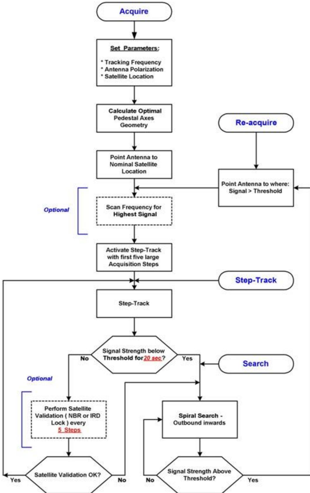
Figure 12.2-1: OceanTRx™ System – Simplified Acquisition and Tracking Algorithm
