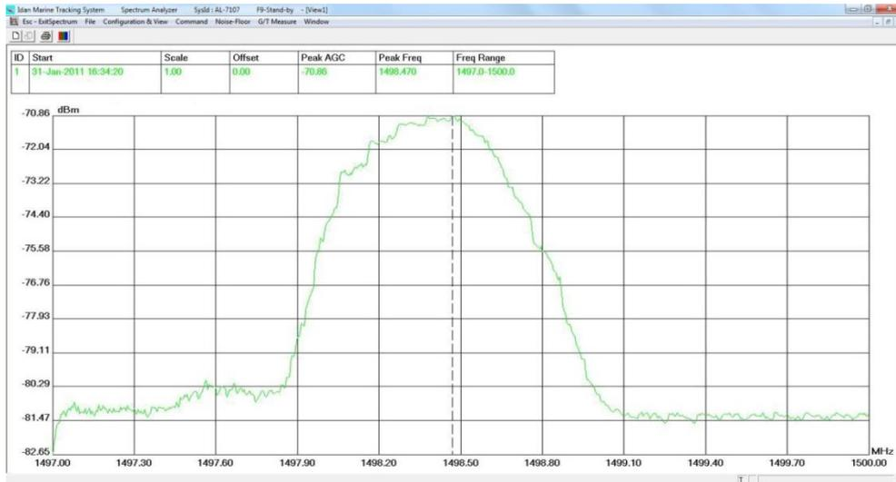
**Figure 12.19-5: MtsVLink Spectrum Analyzer Display with an NBR IfBw of 300 KHz**
