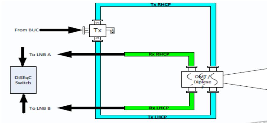
Figure 6.6-2: Feed RF connections
