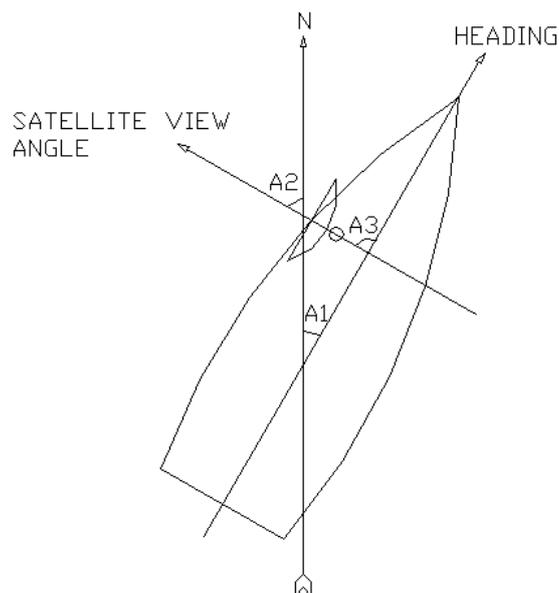
Figure 11.9-1: Blockage Zone azimuth Variables
