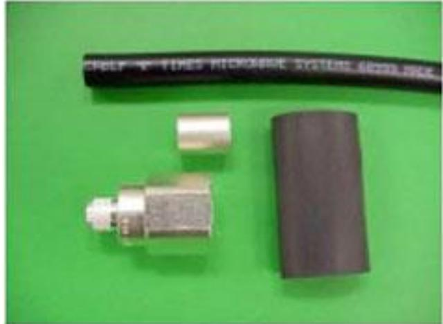
**STEP 2:** Slide the heat-shrink boot and crimp ring onto the cable. Strip the cable end using the ST-400-EZ prep/strip tool by inserting the cable into End 1 and rotating the tool. Remove any residual plastic from the center conductor.
