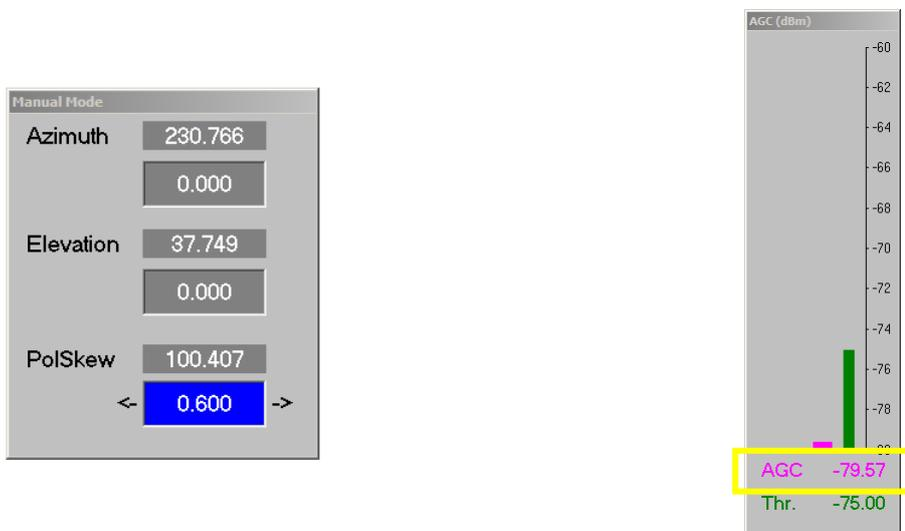
**Figure 11.7-5: AGC Signal received level at X-Polarization after adjustment**
