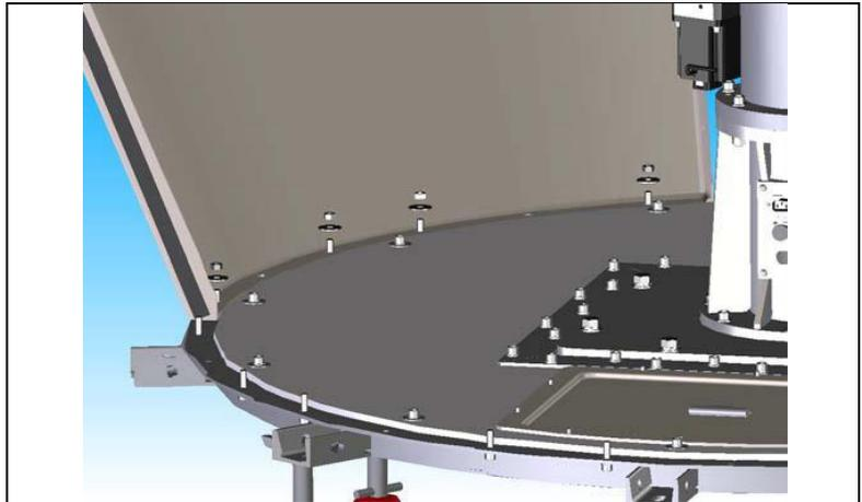
Figure 9.5-1: ADE Radome Petals to Base Ring Assembly I
