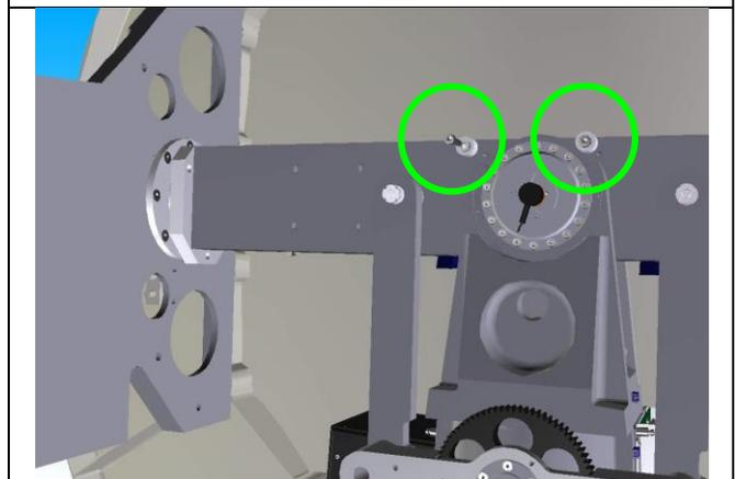
Figure 9.3-2: Tilt Stow Lock Pins
