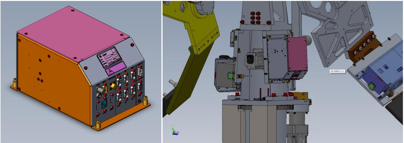
**Figure 6.1-1: Antenna Control Unit (ACU)**
