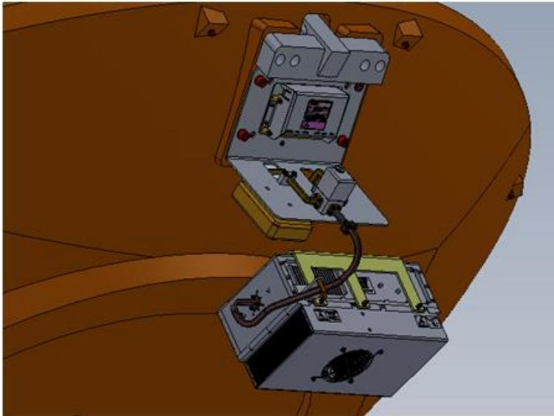
Figure 6.6-1: OceanTRx™7-500 BUC Mounting
