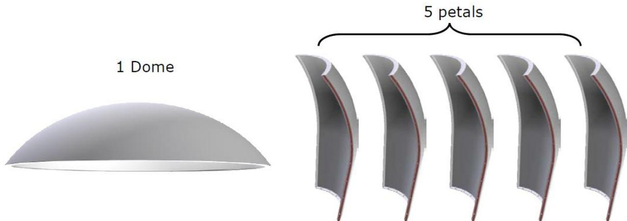
Figure 6.8-1: OceanTRx™7 Radome Elements
