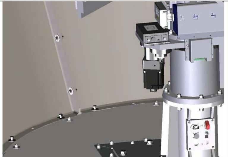
**Figure 9.5-6: ADE Radome Petals to Base Ring Assembly II**
