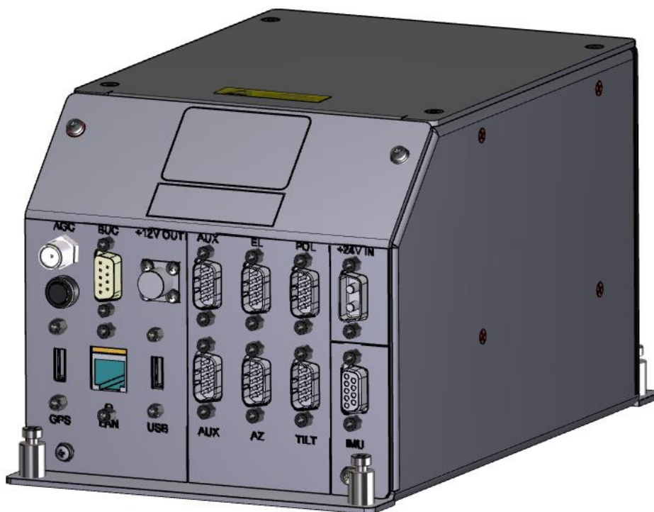
Figure 2-9: Antenna Control Unit
