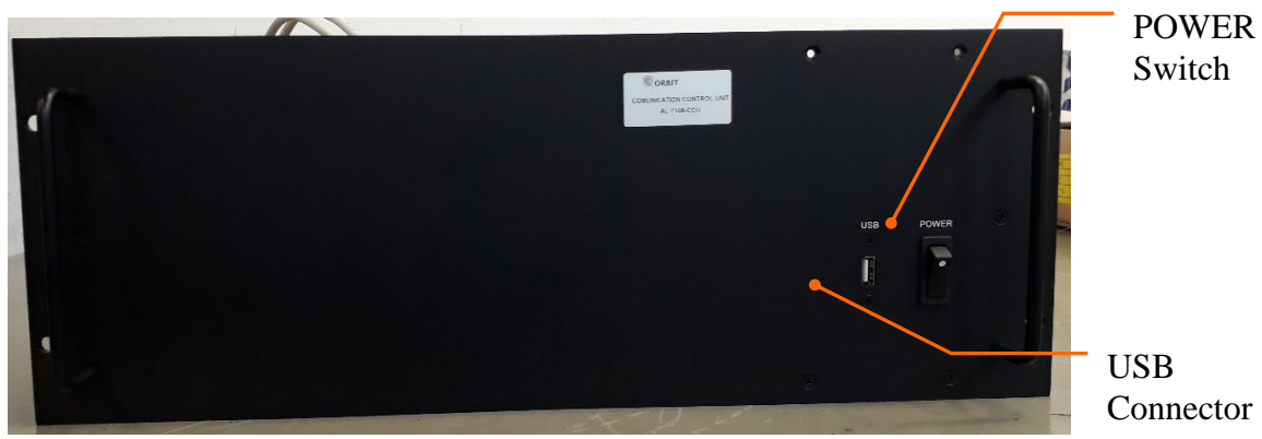
Figure 15. CCU Front Panel
