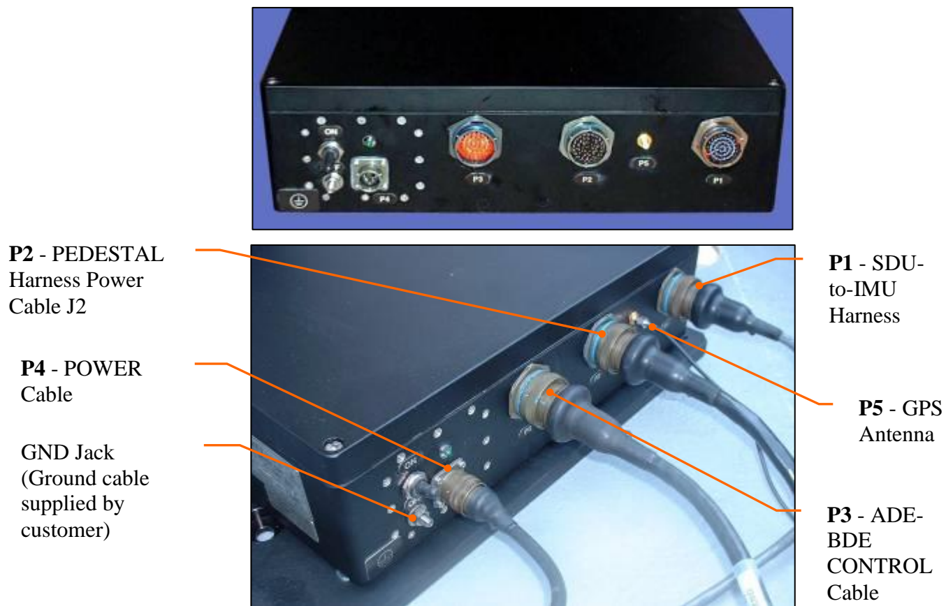
Figure 73. SDU Connectors and Connected Cables
