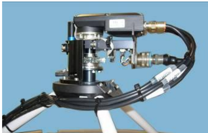
Figure 7-11. Connecting the RF Cables to the Feed
