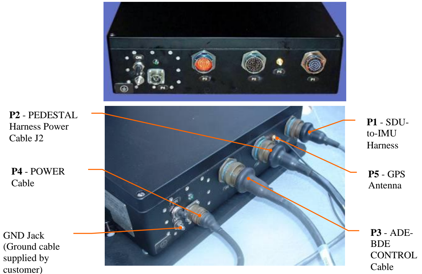
Figure 7-9. SDU Connectors and Connected Cables
