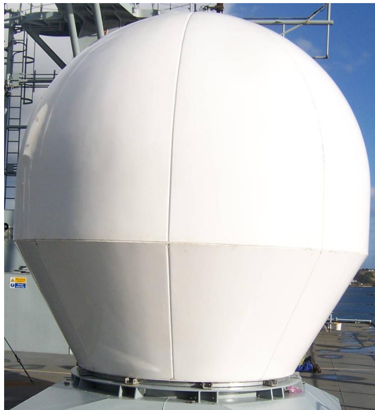
Figure 2-7: Above Deck Equipment (ADE) with Radome
