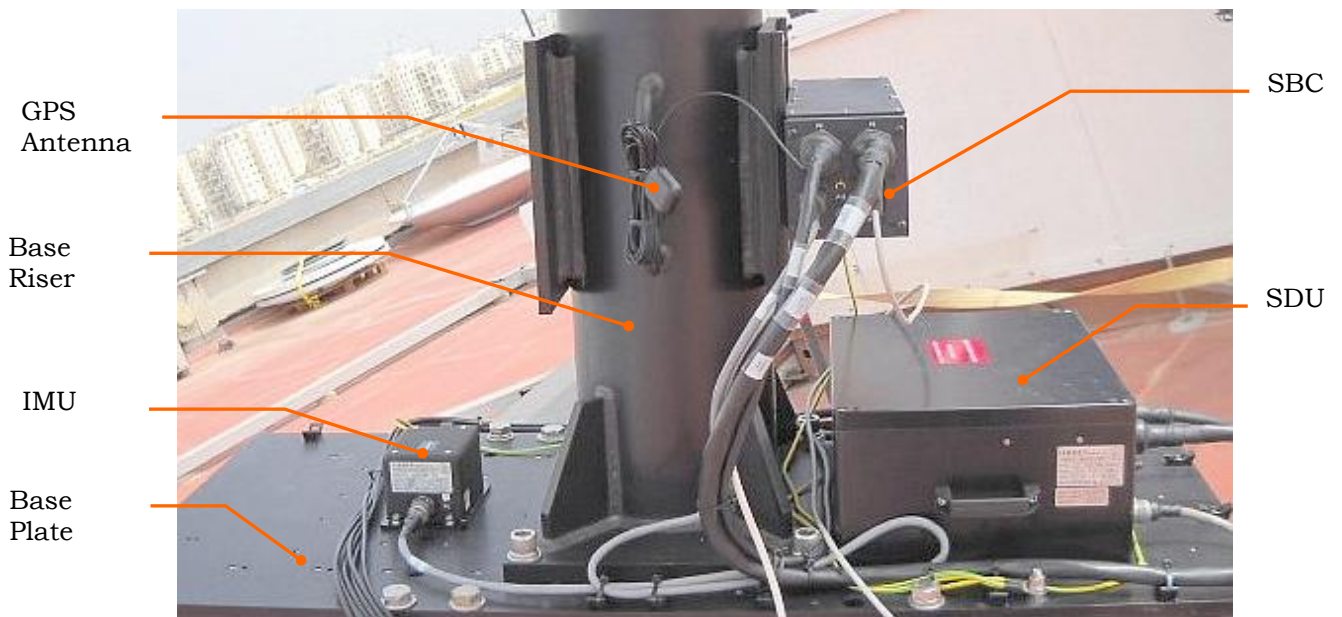
Figure 2-2: ADE Major System Components Location
