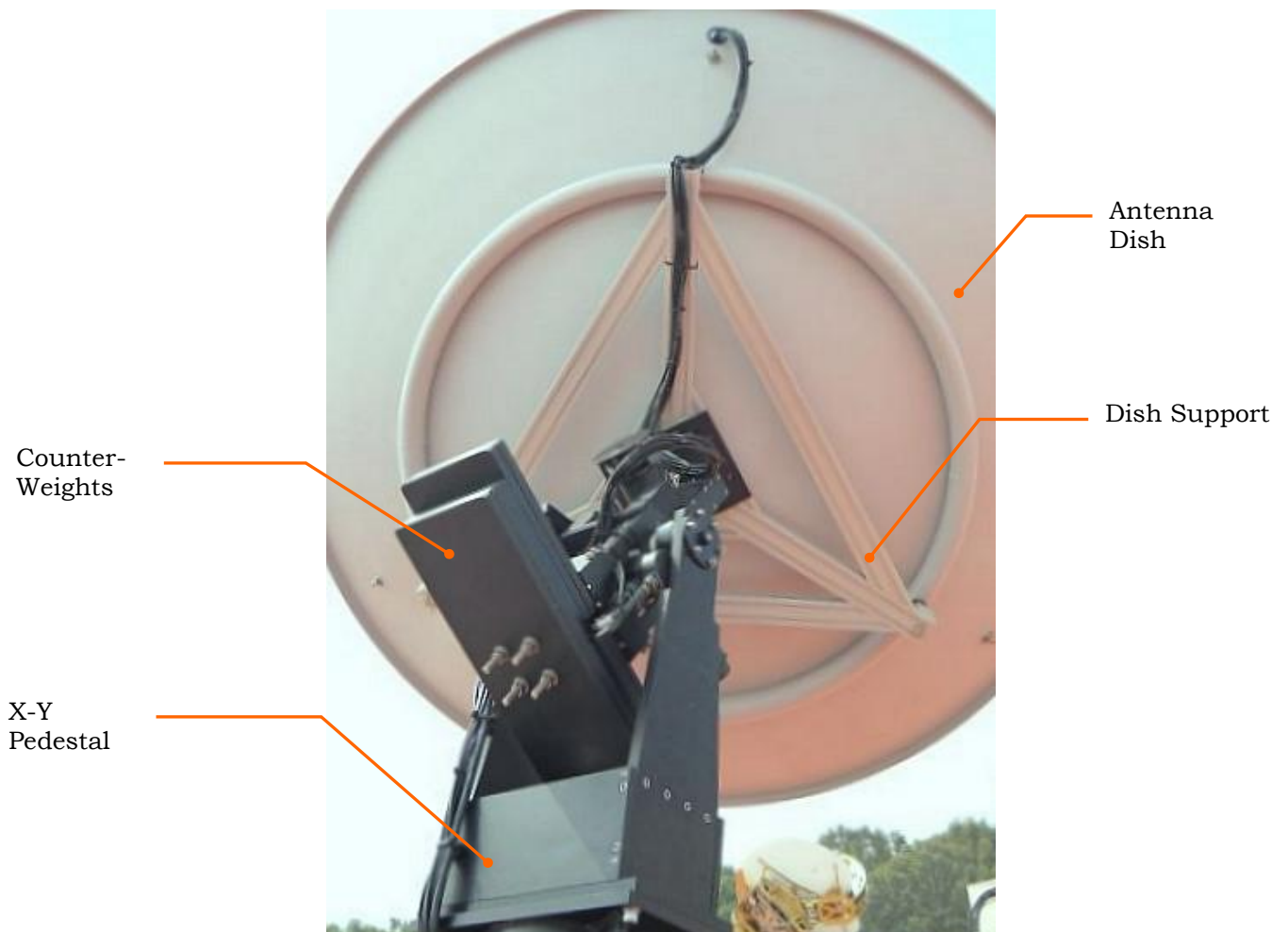
Figure 2-3: Antenna Dish General View
