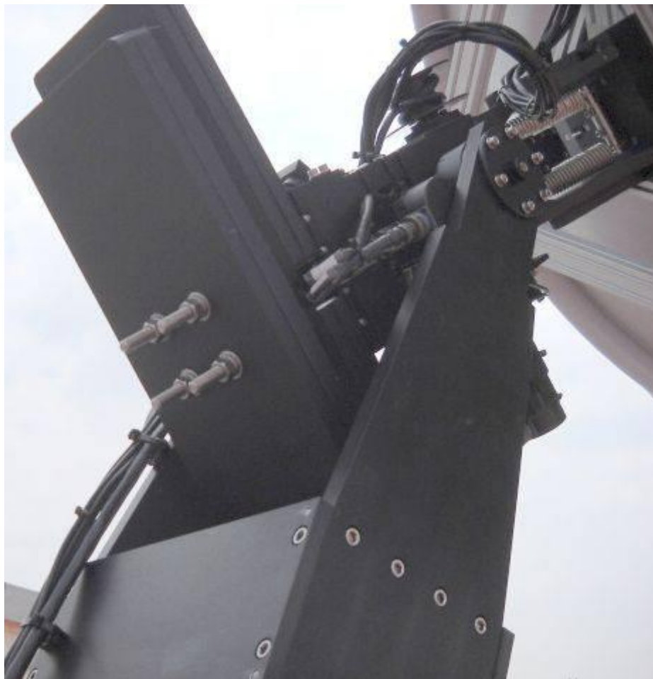
Figure 9-36: Positioner with all the weights installed
