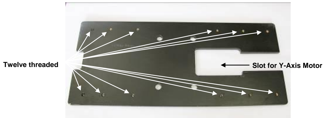
Figure 9-35: Weight with slot and twelve threaded holes
