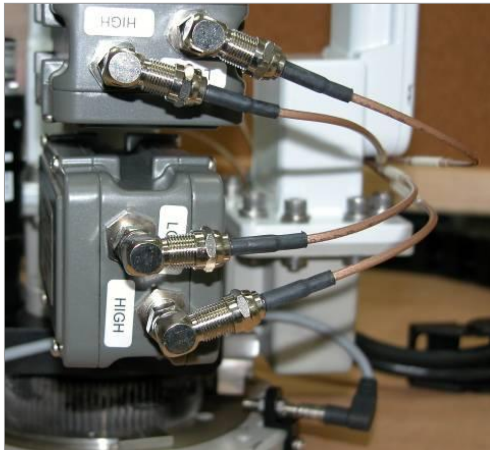
Figure 9-30: KU Band Cable Connections
