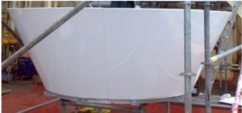
Figure 9-18: Lower Radome Section Secured to Radome Base
