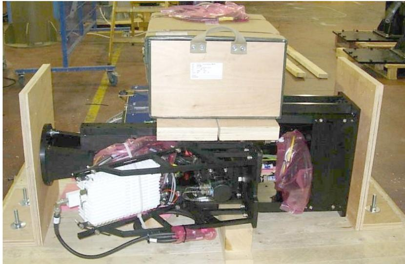
2. Remove all the screws from the holding bracket that secures the PETITIONER'S UPPER MOUNTING PLATE to the shipping crate, stand the POSITIONER on its MOUNTING PLATE and remove the holding bracket from the UPPER MOUNTING PLATE, as illustrated below.
