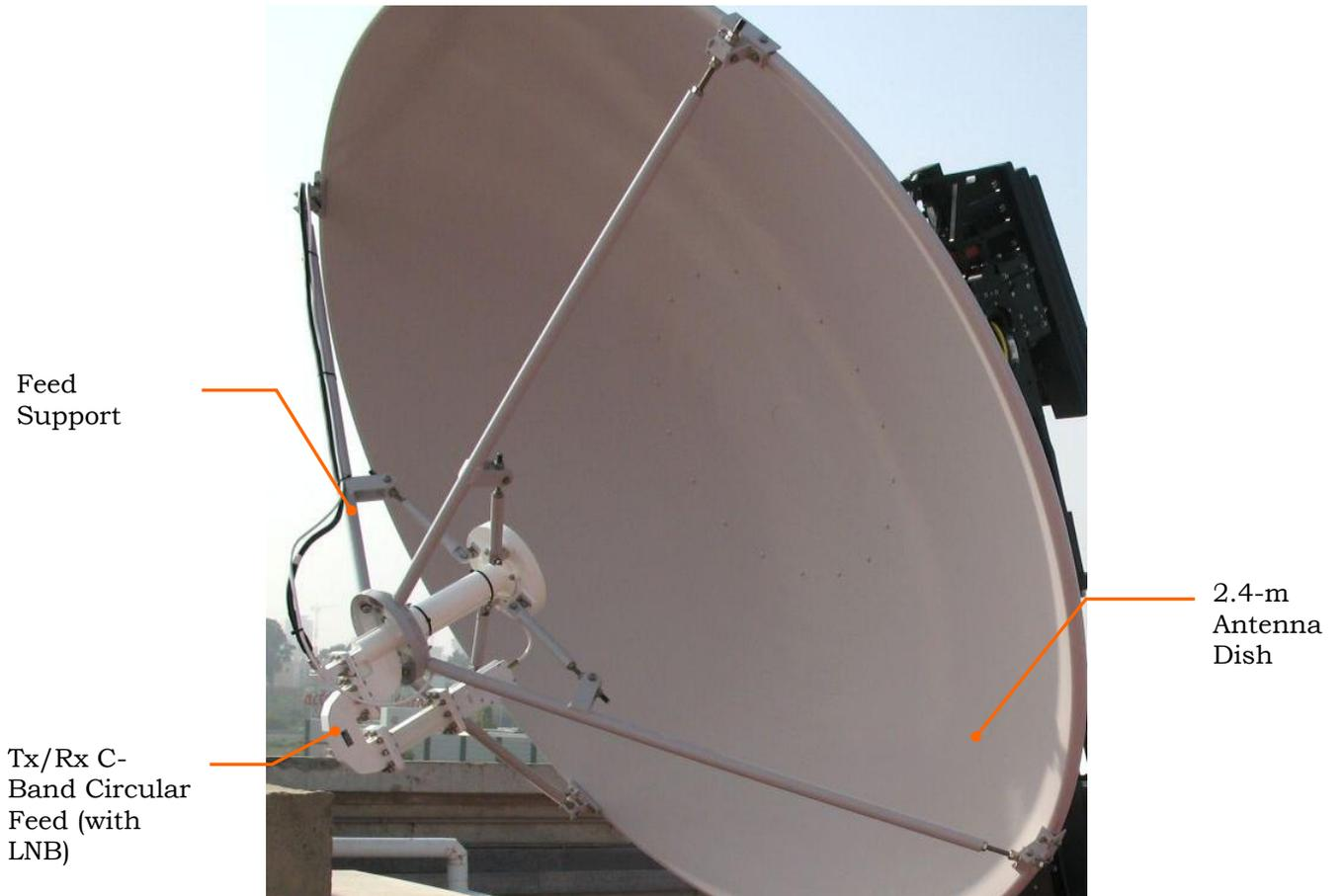
**Figure 2-10:20/40W C-Band Feed General View**
