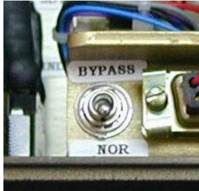
When the system is equipped with an Interlock, setting the switch to the BYPASS position will enable operation when the Radome hatch is open (for maintenance/installation purposes).
