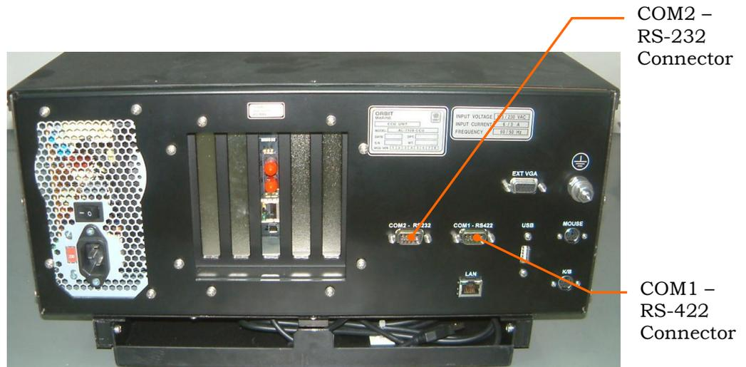
**Figure 10-9: CCU Rear Panel – Serial and Compass Connectors**
