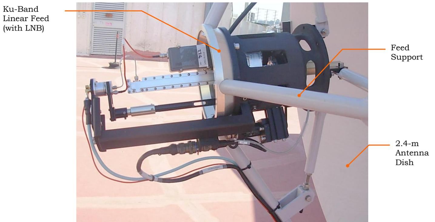
**Figure 2-11:8W Ku-Band Feed General View**
