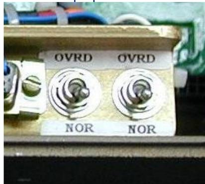
To release the brake of one of the axes, connect power to the SDU (via connector P1), and set the pertaining switch to the OVRD position. This will supply power to the brake and disengage it to allow free movement of the axis. A **Pedestal X/Y brake override** warning will be displayed by the **MTSLink** software on the CCU screen.
