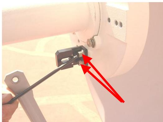
**Figure 12-7: Removing the Feed Bracket (2)**
