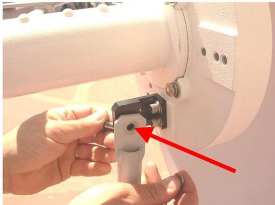
**Figure 12-6: Removing the Feed Bracket (1)**
