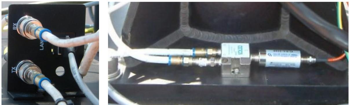
Figure 2-6: Connectors Panel and RF Splitter
