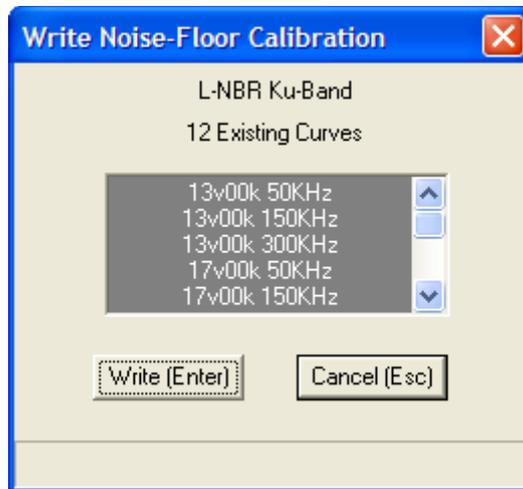
Hit "Write" to save the calibration results in the SBC Flash memory.
