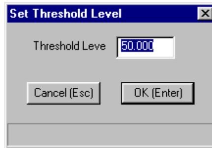
2. Type in a new value (in  $\text{db}\mu\text{V}$ ) into the window, and press ENTER to confirm.
