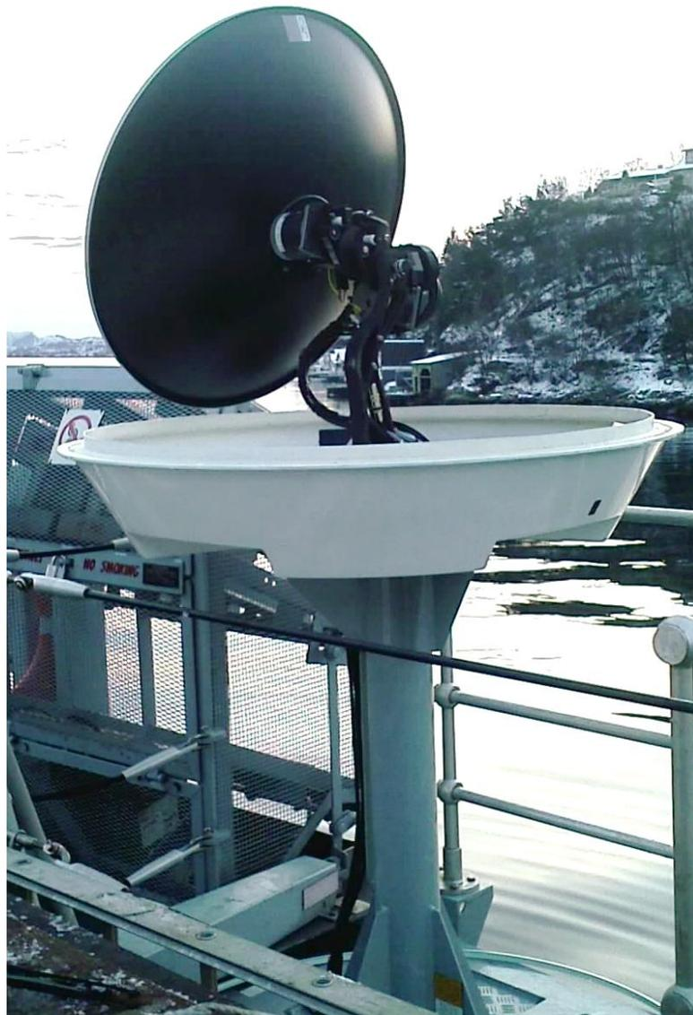
***Figure 2. ADE General View – Radome Removed***
