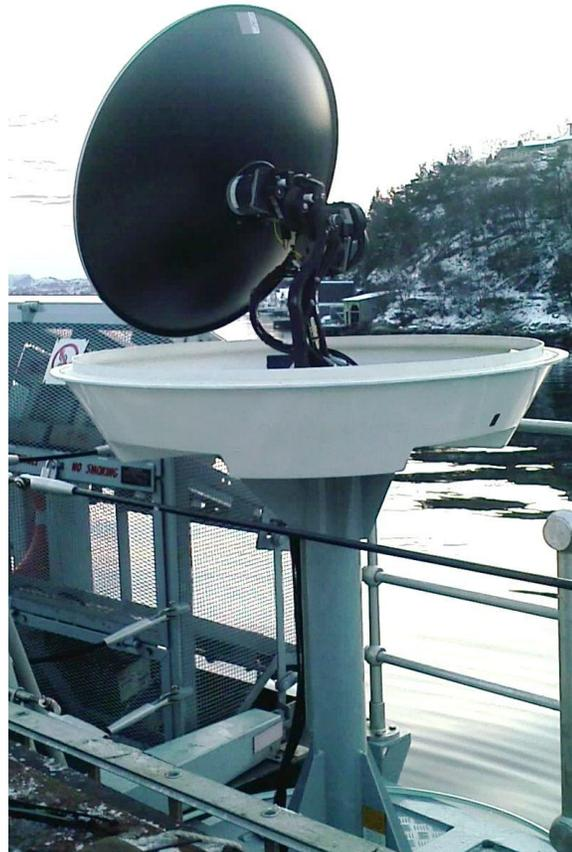
***Figure 39. ADE Base Mounting Orientation***
