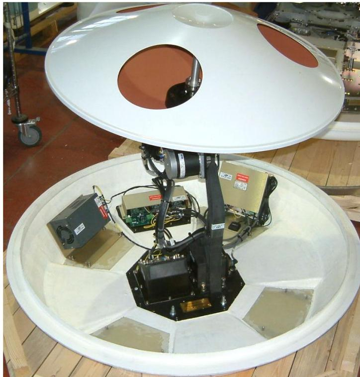
**Figure 3. ADE General Internal View (Radome Removed)**
