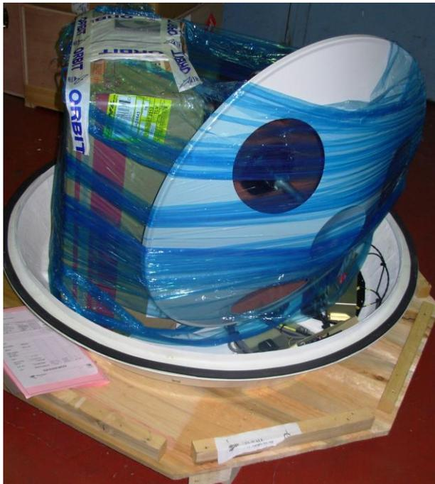
**Figure 37. AL-7203 Shipping Crate- Internal Arrangement (Radome Removed)**
