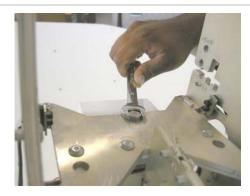
Install the FEED SUBASSEMBLY (1) on the DISH ASSEMBLY.
