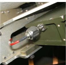
**Step 23**Connect the RF CABLE (12) to the Waveguide-to-Coax connector on the RRF ASSEMBLY.
