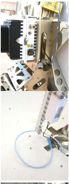
Release the inner and outer nuts and remove the screws and washers.
