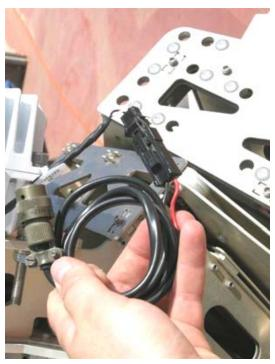
**Step 2**Disconnect the cables from the BUC connectors.
