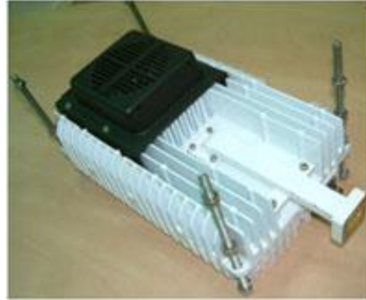
Figure 3-19: 16W BUC (Typical)
