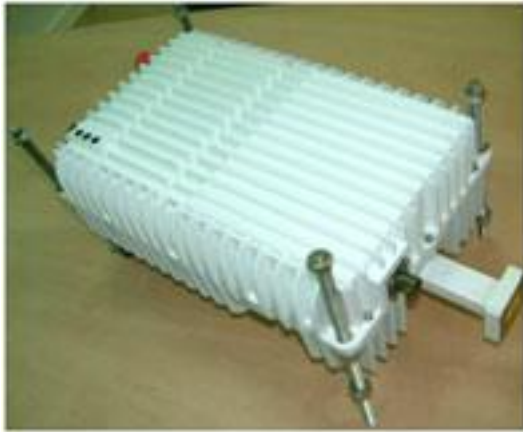
Figure 3-19: 16W BUC (Typical)
