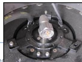
Using a short Philips screwdriver, remove the 3 Philips bolt securing SR-RJ.
